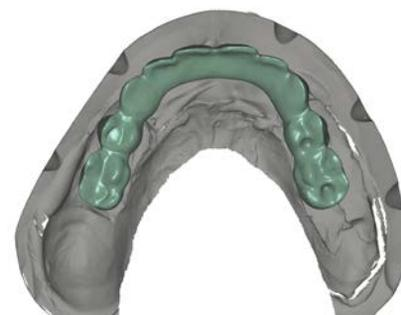
**Figure 19:** Virtual framework before sintering.
