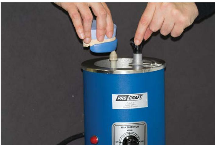
Figure 9: Wax injector.
